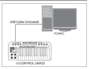
Fig. 1.1: Power supply via USB
